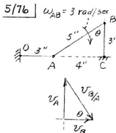
$$v_B = v_A + v_{B/A}, \quad \omega_{BC} = \frac{v_B}{BC} \quad -۵$$
