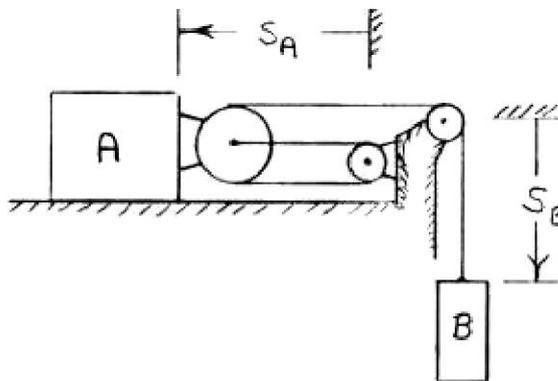
$$\text{Length of cable } L = 3S_A + S_B + \text{Constant}$$
