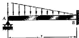
Reactions are statically indeterminate.
