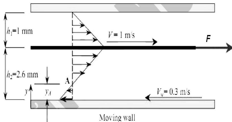
(b) The magnitudes of shear forces acting on the upper and lower surfaces of the plate are
