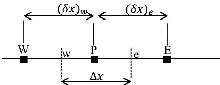
$$\frac{d^2T}{dx^2} = \frac{2}{(\delta x)_e + (\delta x)_w} \left[ \frac{T_E - T_P}{(\delta x)_e} - \frac{T_P - T_w}{(\delta x)_w} \right]$$
